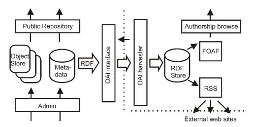
Fig. 1. A schematic of the repository emphasizing the RDF module components.
